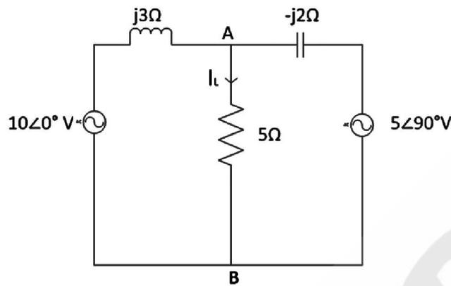
11. Calculate the loop currents using graph theory.
